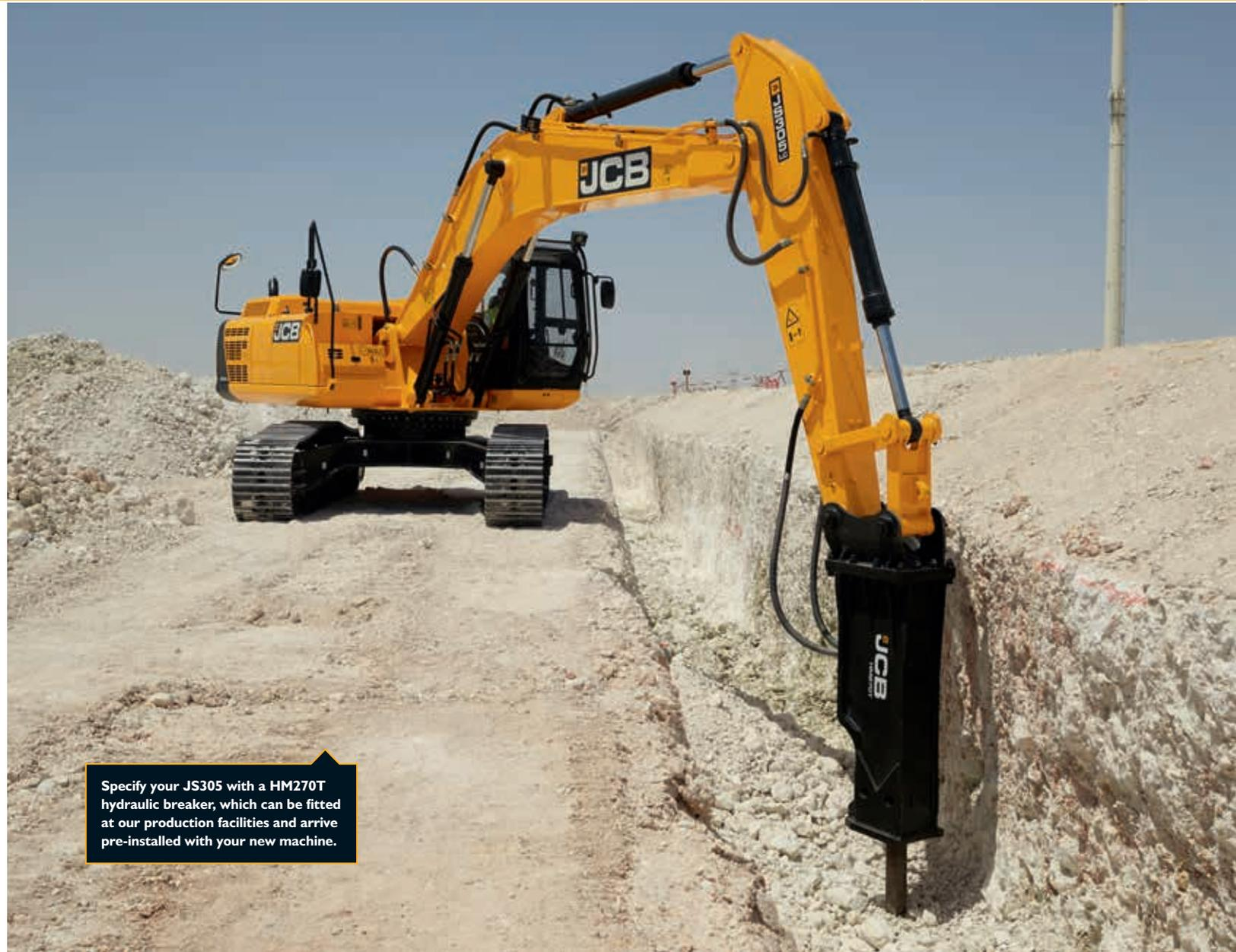
Specify your JS305 with a HM270T hydraulic breaker, which can be fitted at our production facilities and arrive pre-installed with your new machine.
